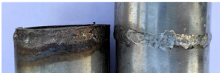
Figure 8.1: Oxidation of Stainless Steel Weld Metal
