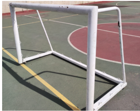
Figure 9.21: Locations Where L Elbows Are Used
