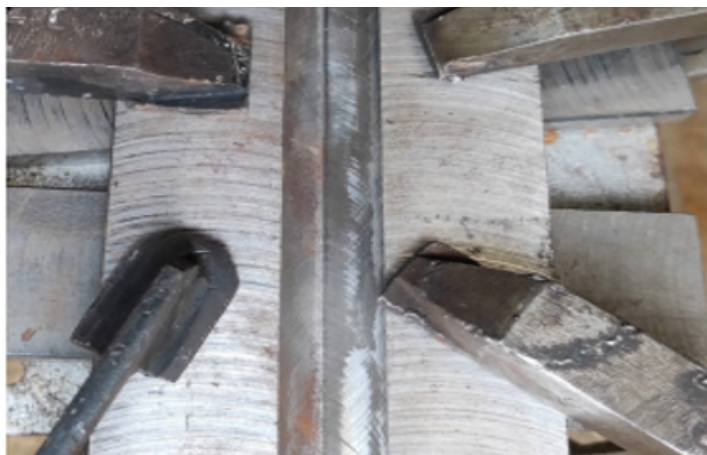
Figure 1.7: Preventing Weld Shrinkage Using a Fixture.
