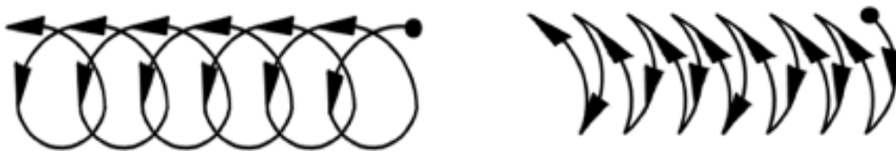
Figure 1.16: Recommended Electrode Movements for Fill Passes
